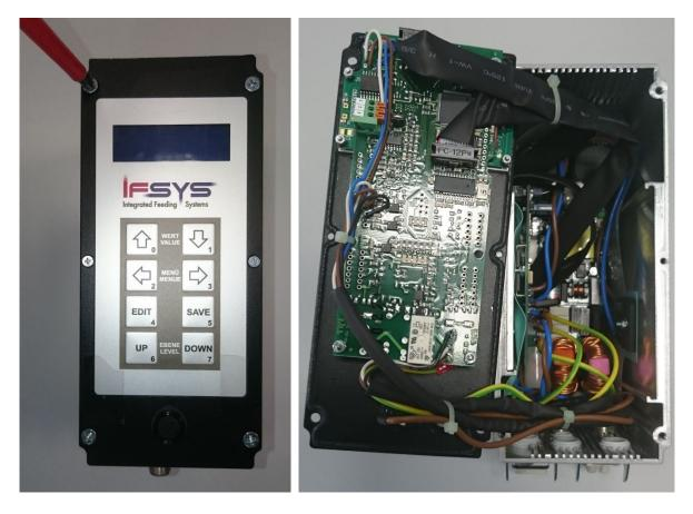
When closing the cover of the enclosure, make sure that no cables are caught in it. Position the cover back on the enclosure and secure it with the removed screws.
